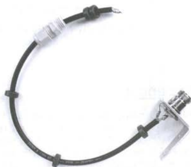
Pc. 10: Photo of quarter wave sleeve of RG58 as used in measurements
