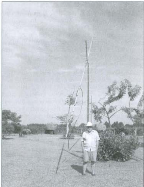
OA4TT: on 2m EME from Peru using a proven DJ9BV design on a long bamboo boom
