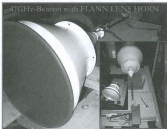
Fig. 10: Beacon with Flann lens horn antenna
