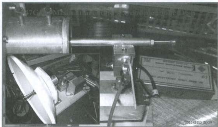
Fig. 8: Assembled combination of mixer, circular WG and feed
