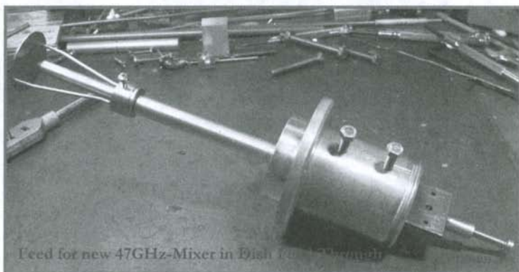
Fig. 9: Combination of circular WG, dish feed and mixer on test in dish feed trough. The 25cm aluminium tube (WG for 23.5GHz) was shortened later on.
