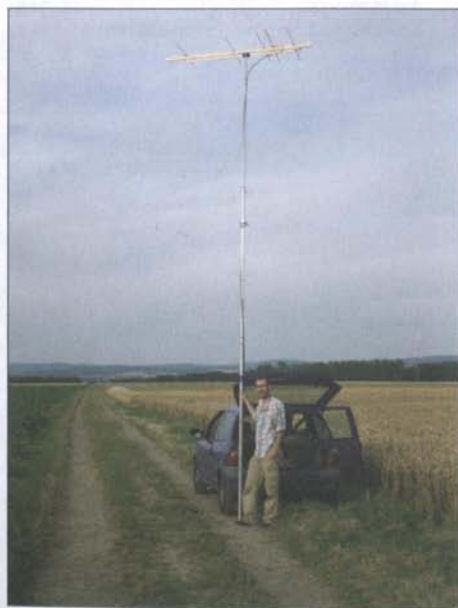
Pc. 4: Measuring the wooden boom version with insulators #23040.20 and M3 screws
