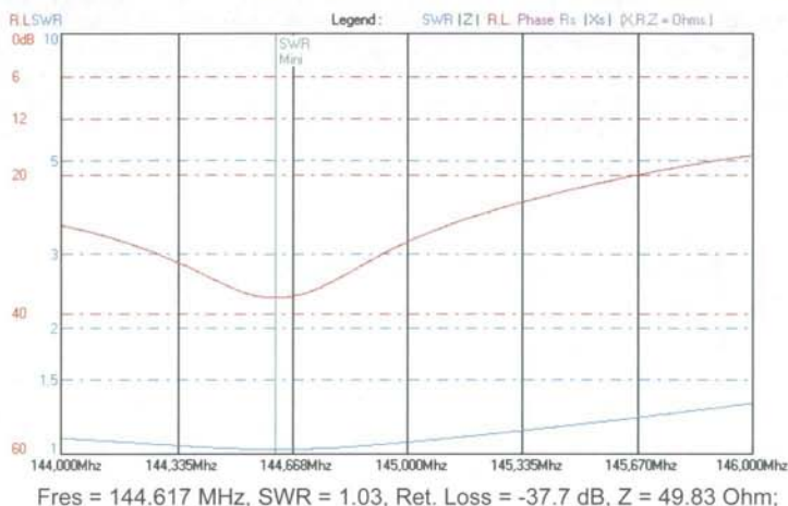
Chart 2: Measured plot of the wooden boom Yagi with zero BC
