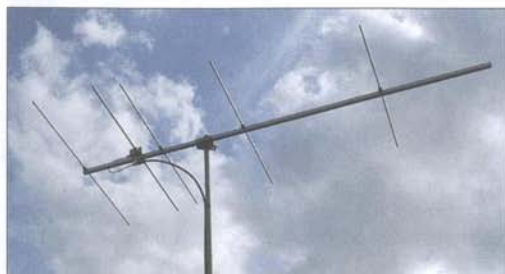
Pc. 5: With BC of 2 x 5 = 10 mm on 20 x 20 mm aluminium boom and insulators #23040.20
