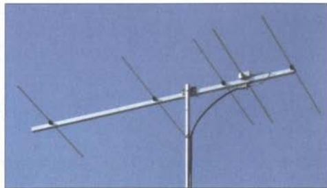
Pc. 5: With BC of 2 x 5 = 10 mm on 20 x 20 mm aluminium boom and insulators #23040.20
