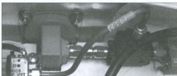
Fig. 8: Close up of the circulator/transition output network
