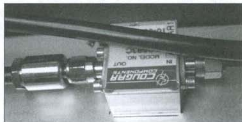
Fig. 9: Close up of the Cougar 5-1000MHz broadband IF amplifier
